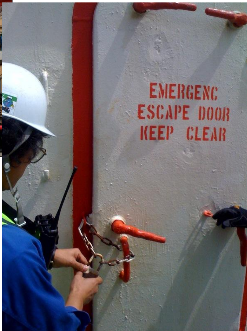
Top: Port State Control team is challenged by gangway watch, upon arrival at vessel (USCG Sector Anchorage) Right: Improperly secured and labeled escape door, (USCG Sector Puget Sound).
